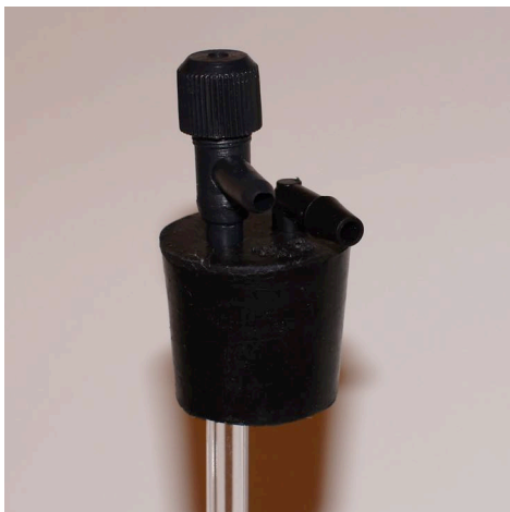
Figure 2 – Rubber Stopper with air valve and drain elbow
