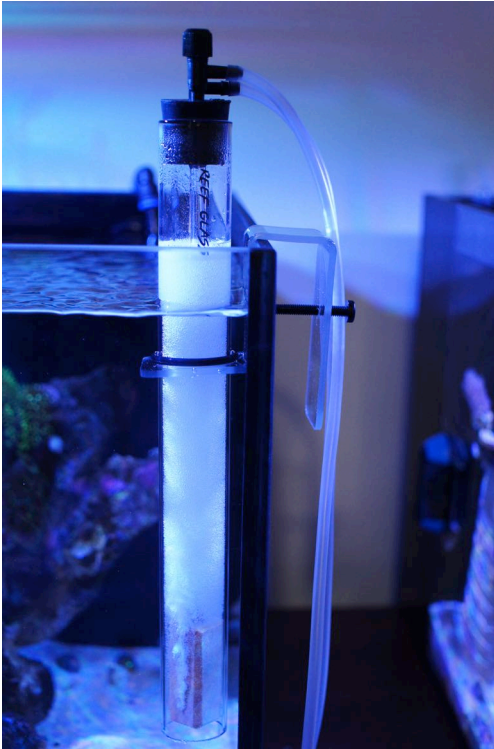
Figure 7 - Skimmer with abundant micro-bubbles
